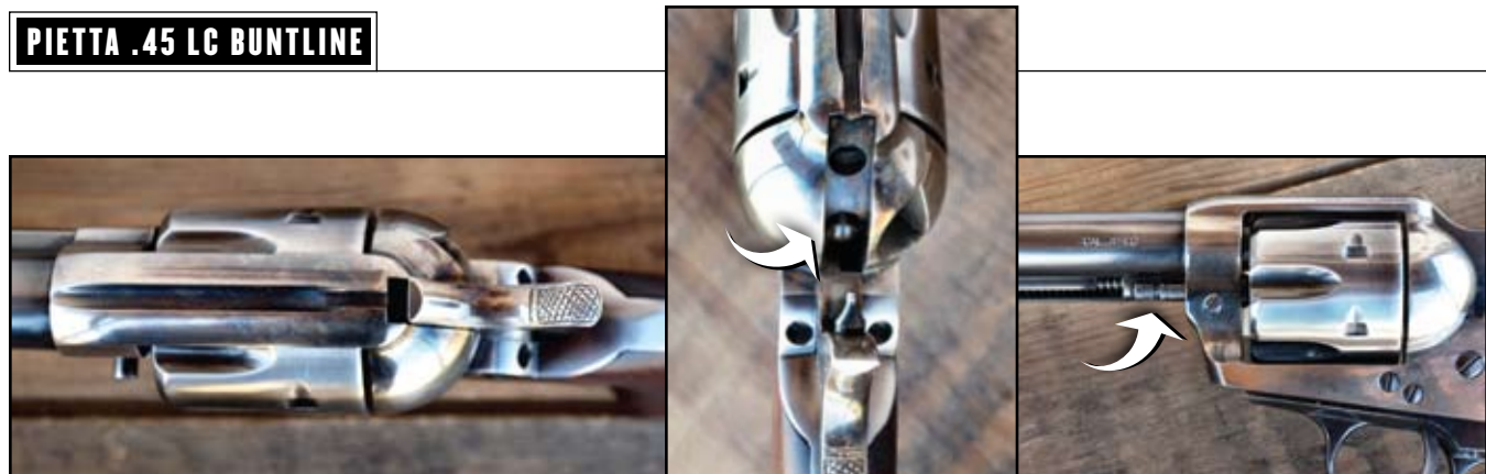
Pietta uses a double notched cylinder arbor and the transverse latch to create a safety mechanism. By depressing the latch and pushing the cylinder arbor further back, the rounded end protrudes through the back of the frame (arrow) blocking the hammer from fully dropping into battery.
